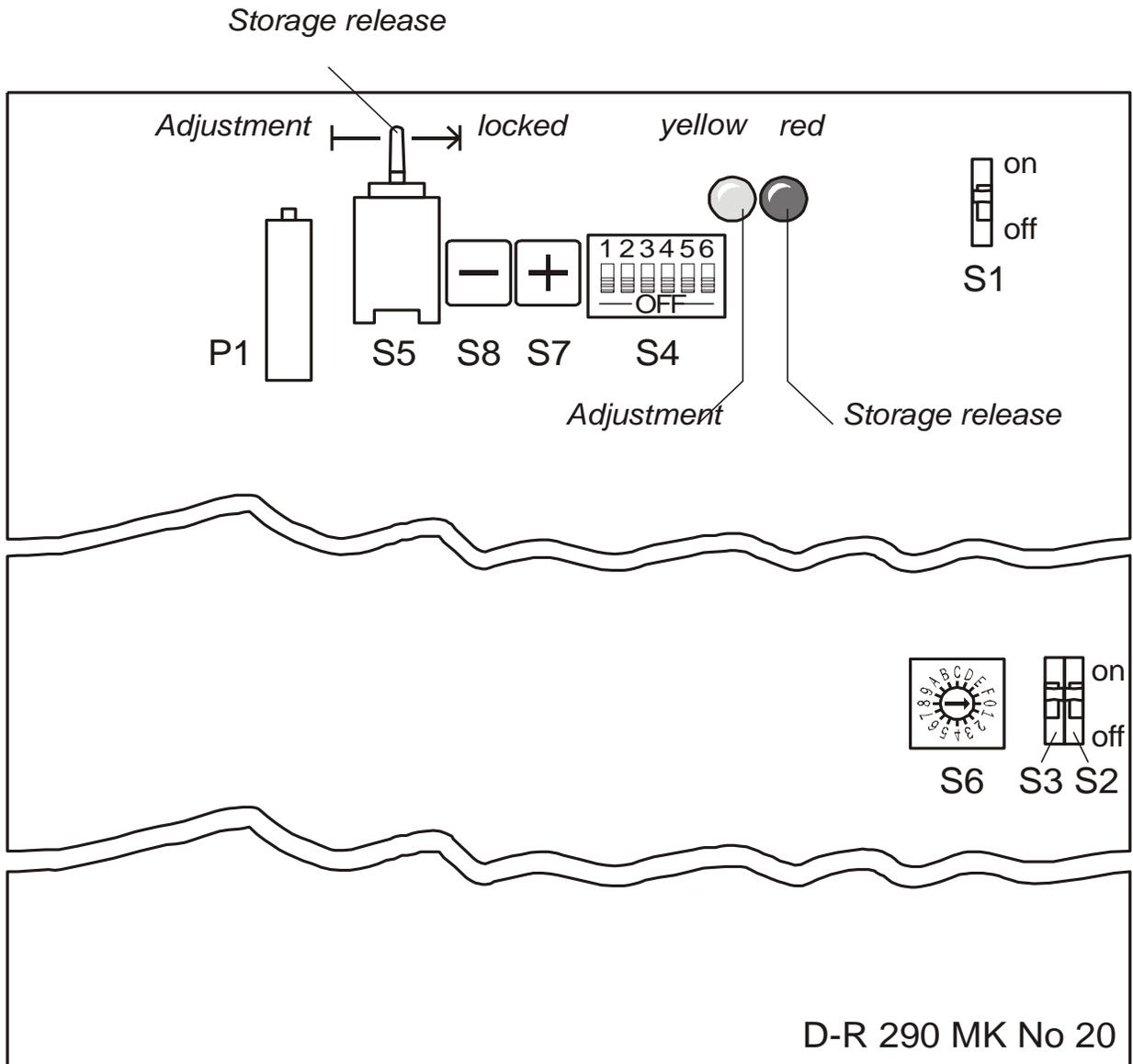
(Fig. 6.5) Transceiver switch functions
