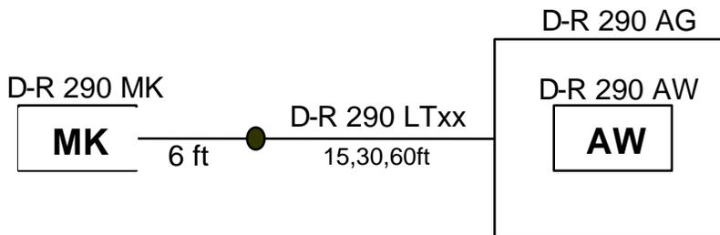
Similar to above except an extension cable is placed between transceiver and **D-R 290 AW**.
