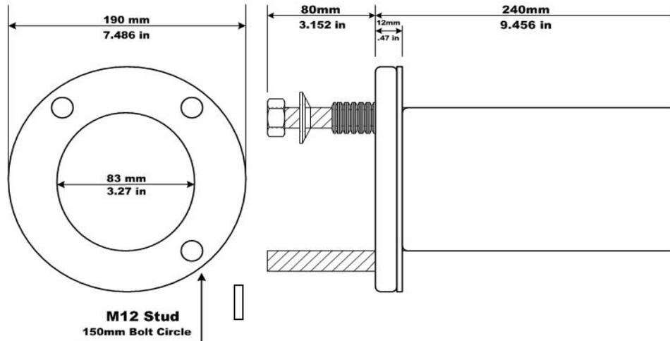
(Fig. 5.1) D-R 280-10E installation flange for D-R 290 Opacity Monitor
