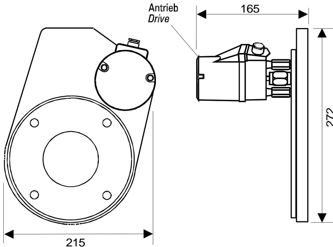
(Fig.9.1 ) Dimensions (in mm) of shutter (D-SK 280 MA)
