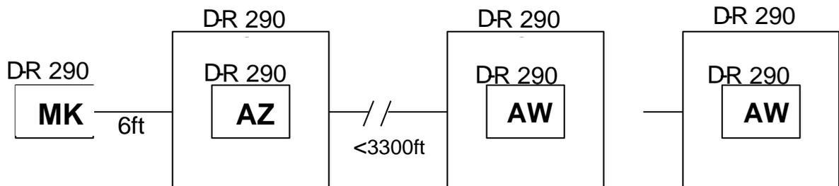
The above diagram shows the recommended mounting arrangement. The **D-R 290 AZ** is used in the **D-R 290 AG** housing at the transceiver location. Calibration functions and filter audits can be ran from this location using the **D-R 290 AZ**. The remotely mounted **D-R 290 AW** can be mounted in the wall mount or panel mount housing with panel mount in a 19" rack being the most common.
