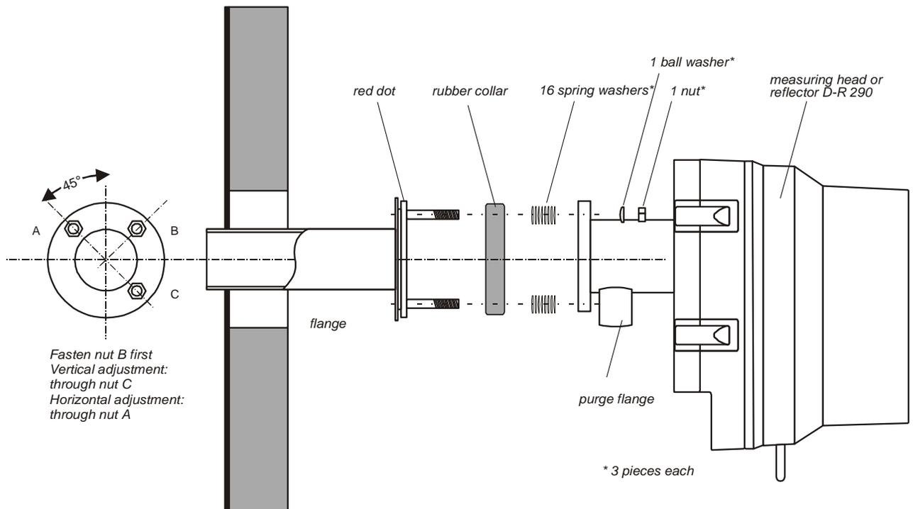
(Fig. 5.7) Mounting monitor on the installation flange
