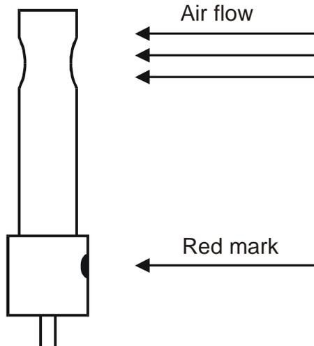
The air current sensor should be mounted on the system after removing the cover (PG7). The sensor should be positioned at the monitor opening such that the air current flows directly through the hole in the sensor. The red mark is meant to aid in mounting and should face away from the monitor in the direction of the air current.
