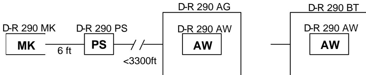
The transceiver is now powered from the **D-R 290 PS** power supply located at the monitor location. Now the **D-R 290 AW** can be located up to 3300 feet (1000m) from the transceiver. A 2 pair cable is used to transmit the data over the RS 422 interface. Since the **D-R 290 AW** unit can be mounted indoors now, a panel mount housing, **D-R 290 BT**, can be used. More information is given on these different housings in the installation section of this manual.
