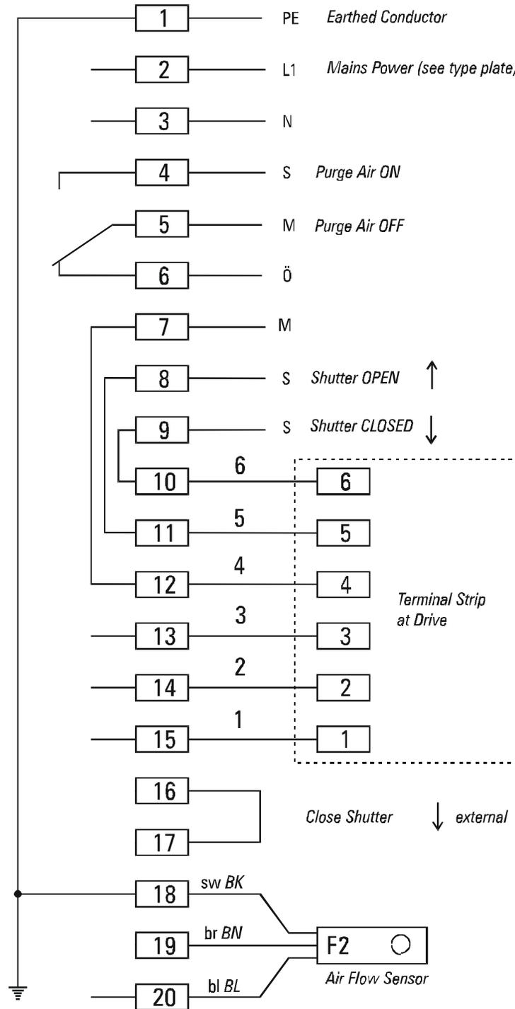
(Fig. 9.5) Electrical Connection for the D-SK AE
