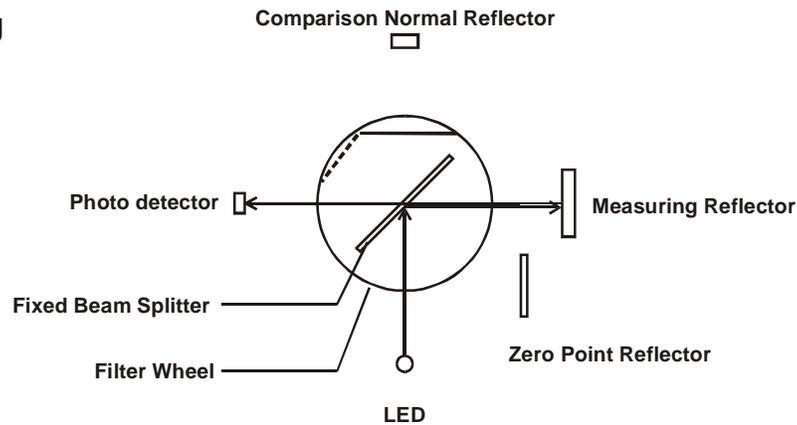
The unavoidable drifts in light intensity that result from aging of the light source or temperature changes are automatically compensated by the monitor. The 2 kHz modulated light is split into both a measurement light beam and a comparison normal. An optical receiver (photo element) alternately reads these light beams. The selection of the light paths is driven by a stepper motor.
