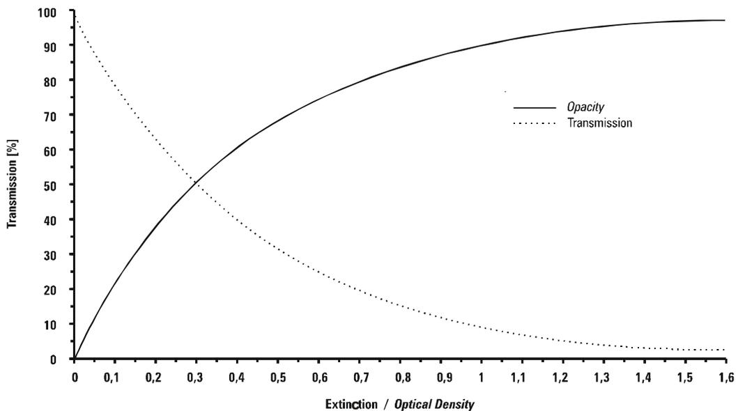
(Fig. 3.1) Relationship between Extinction, Transmission and Opacity
