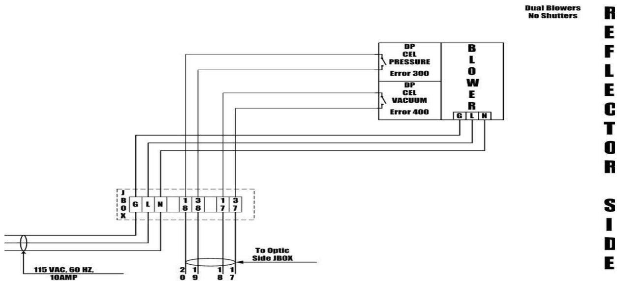
(Fig. 5.4) Reflector side interconnect wiring, typical
