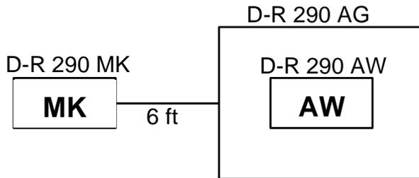
Transceiver connected directly to the **D-R 290 AW** located at transceiver location. The **D-R 290 AW** electronic insert is mounted in the **D-R 290 AG** wall mount housing.
