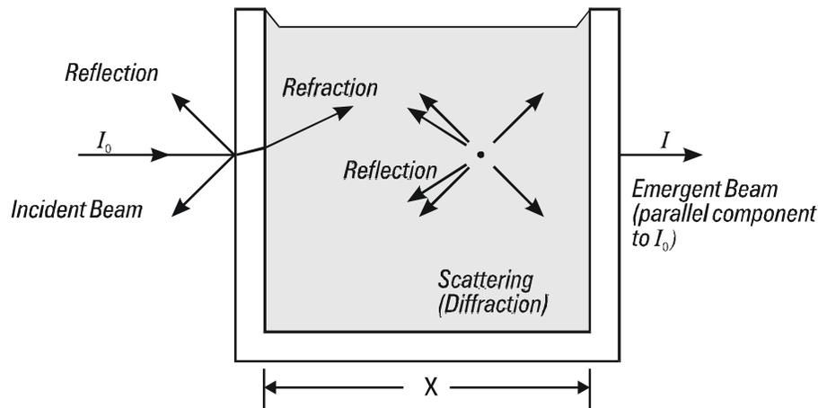
The light beam loses intensity proportionally to the particle concentration of the air. The light beam has a significantly larger diameter than the reflector surface. This makes alignment easier and reduces measurement errors caused by possible heat-induced shifts in the transceiver or reflector mounting flanges.
