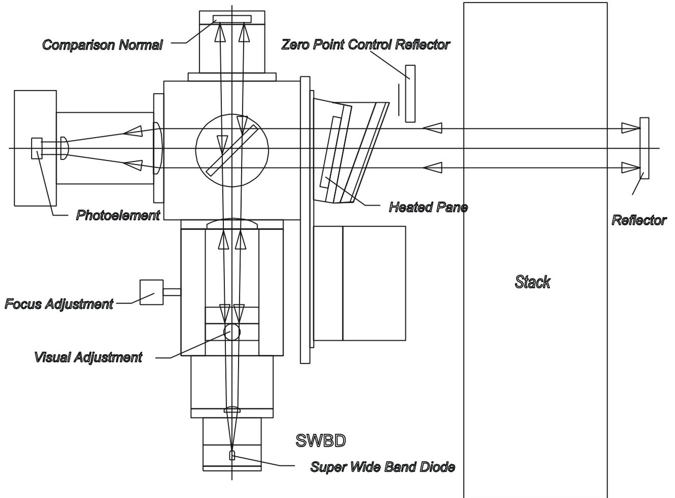
(Fig. 3.3) Optics diagram D-R 290
