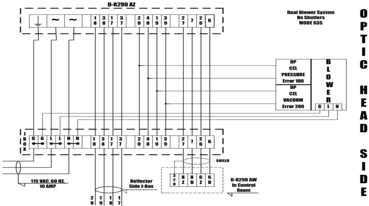
(Fig. 5.3) Transceiver side interconnect wiring, typical
