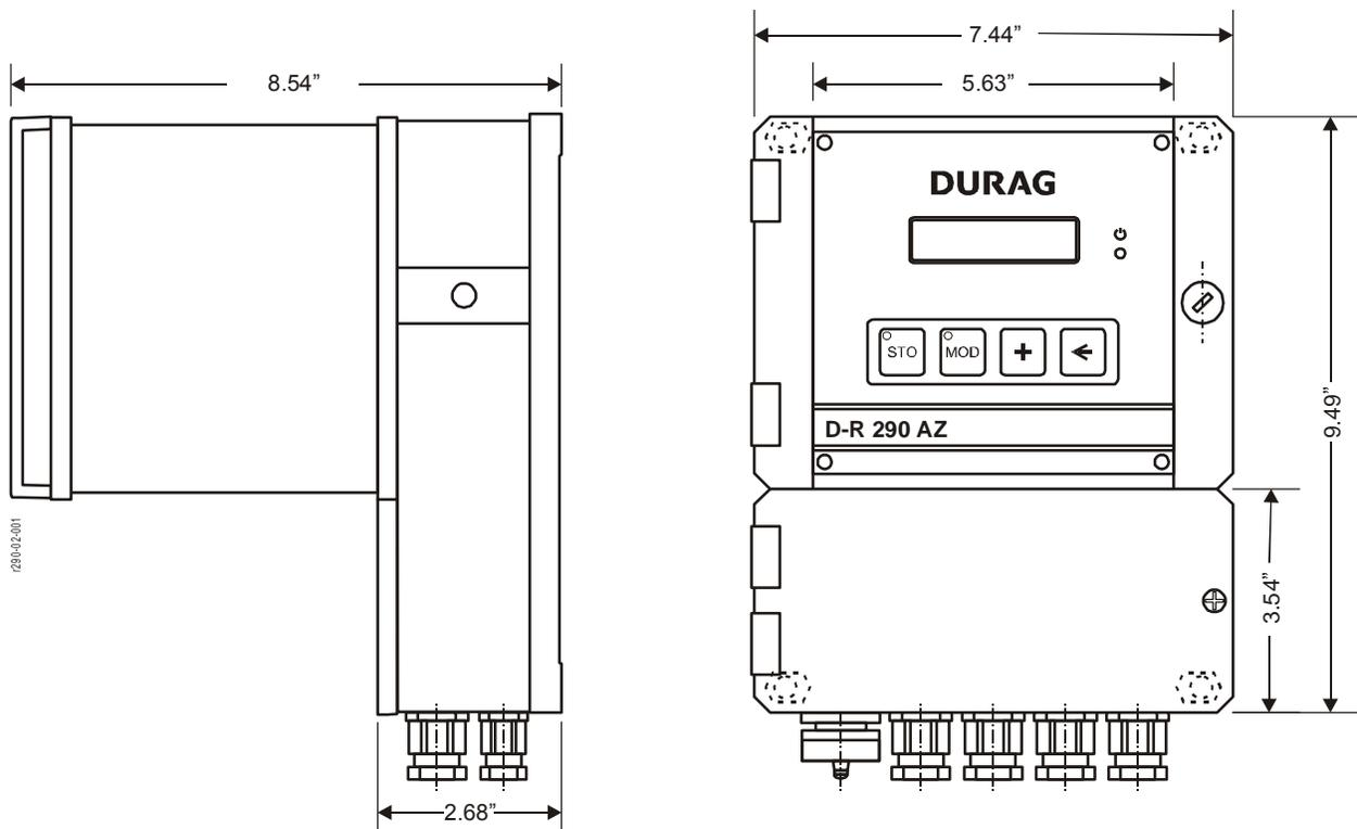
(Fig. 5.5) D-R 290 AG wall mount housing dimensions
